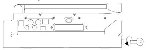
There is 2 PCI slots on the Dockunder. Maximum card dimensions are 260mm (L: length, including L-bracket thickness) x 115mm (W: width, including gold fingers) x 25 mm (H: height). The total power rating of 2 PCI slots is +5V 3A, +3.3V 3A, +12V 300mA, -12V 300mA.
